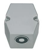
The LCN SEM7800 Series are heavy duty, electrically controlled door holding magnets. Magnets are fail safe and hold until the current is interrupted. A manual door closer is used to control and close the door. A choice of floor, recessed wall, or surface mounted wall magnets are available.
